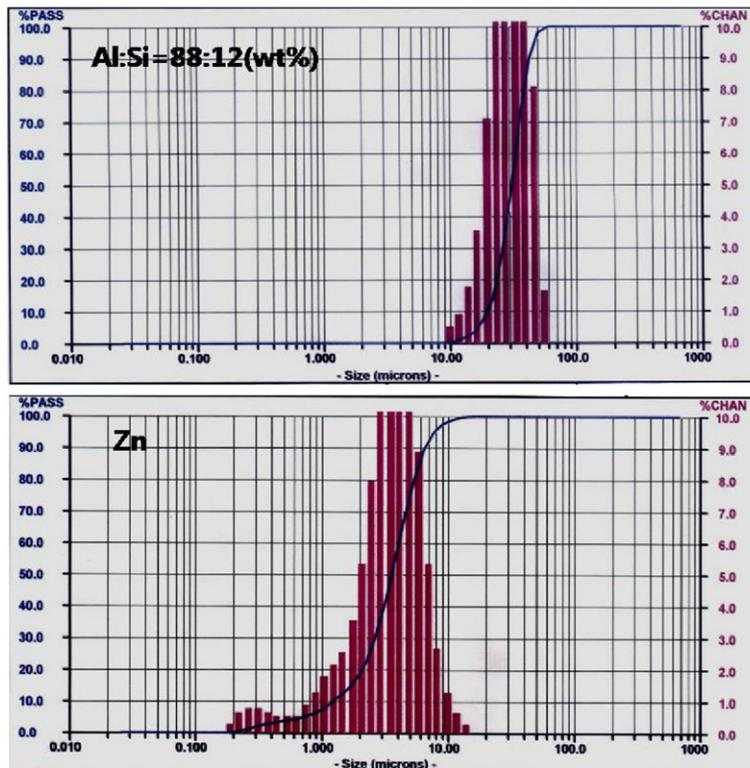
(b) Laser scatter value of Al-Si and Zn powder size distribution (volume fraction)
