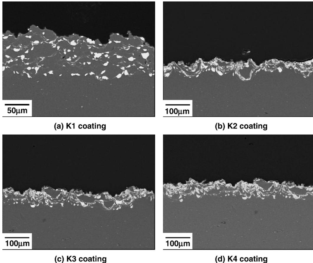
Fig. 4. The cross-sectional microstructures of the as-sprayed coating.
