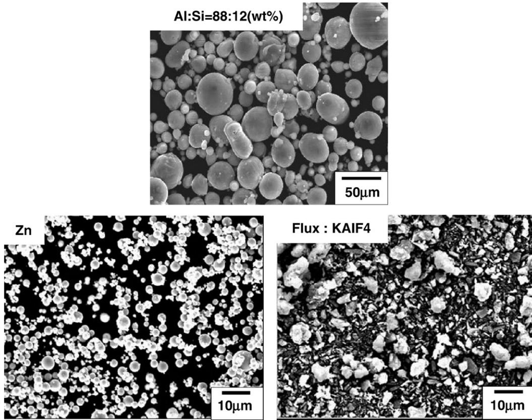
(a) SEM micrograph of Al-Si, Zn and flux powder morphology
