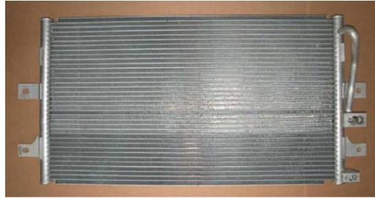
**(a) Leak test before the corrosion test**
