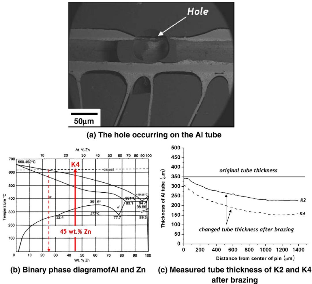
Fig. 7. The effect of zinc content on aluminum tube thickness after brazing.
