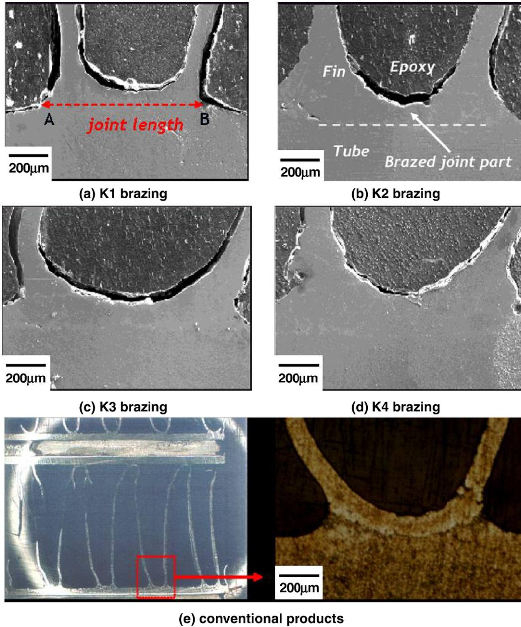
Fig. 5. Cross-sectional microstructures of the joint after brazing.
