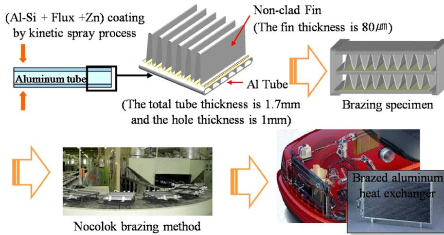
Fig. 1. Schematic process of the brazed aluminum heat exchanger manufacturing using kinetic spraying process.
