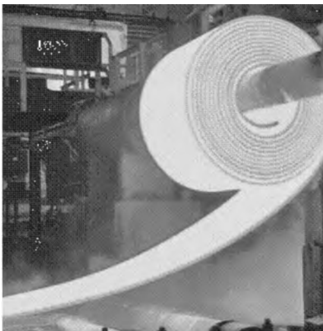
Fig. 2 Hot steel coil being wound, showing the harsh conditions of steel manufacturing
