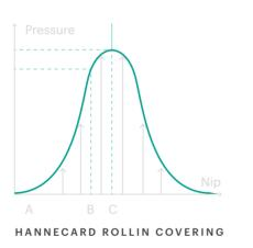
Furthermore, Hannecard Rollin combines specific properties of their covers with an optimized nip calculation. This allows the paper converter to obtain the required thickness, without having to press harder on the embossing roll.
